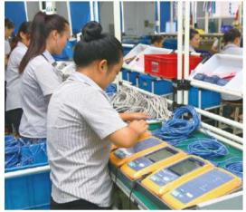
100% FLUKE Component Test for Patch Cord
